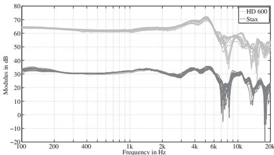
**Figure 2:** HpTF of two open-type headphones measured with a dummy head. 18 fittings are shown for Sennheiser HD 600 (light gray) and Stax SR Lambda (dark gray, values shifted -30 dB for clarity).
