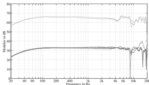
**Figure 7:** Equalization response for two subjects using an individual filter. The light gray curves were generated with the filter shown in Fig. 5. Dark gray curve is shifted -30 dB for clarity.
