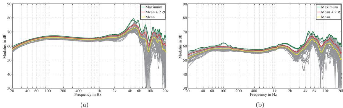
**Figure 4:** Individual HpTF measured at 15 subjects (4 repetitions). Subjects should place the headphone at its most comfortable fit. Left speaker of (a) Sennheiser HD 600 and (b) Stax SR Lambda.
