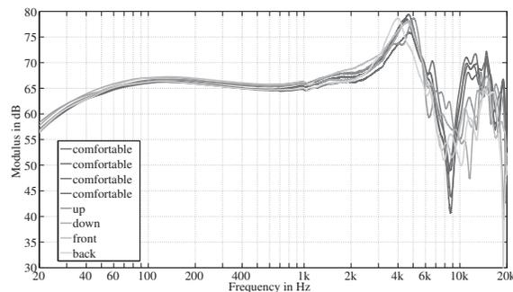
**Figure 3:** HpTF of a single subject measured four times with comfortable fit and at four extreme positions with the Sennheiser HD600 headphone.
